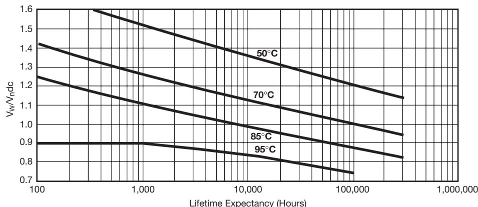
V<sub>w</sub>: permanent working or operating DC-voltage.
