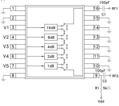
DC blocking capacitors C1 & C2 are required on RF1 & RF2. Choose C1 = C2 =  $100 \sim 300$  pF to allow lowest customer specific frequency to pass with minimal loss. R1 = 5K Ohm is required to supply voltage to the circuit through either PIN 9 or PIN 16.
