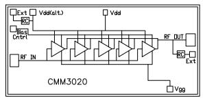
pHEMT is controlled to maintain correct drain current and thus drain voltage. The typical gate voltage needed to do this is 0.5V. Typically the gate is protected with Silicon diodes to limit the applied voltage. Also, make sure to sequence the applied voltage to ensure negative gate bias is available before applying the positive drain supply.
