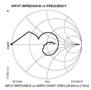
Note: All measurements performed on Hewlett Packard 8753D Network Analyzer (201 sample points, linear scale) in a 50 ohm coplanar waveguide environment. Tables created using MDS software.
