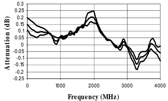
**Typical Attenuation Deviation vs. Temperature for 8 dB Bit**
