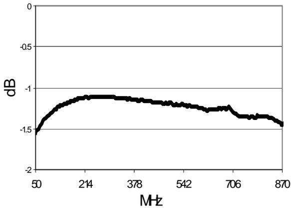
Insertion Loss 2 (Coupled pin 5 to pin 3)
