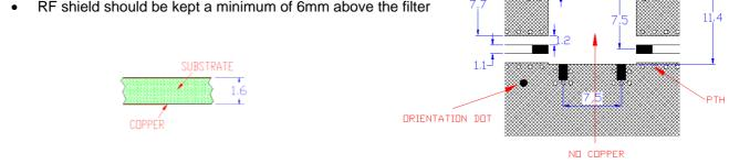
Dimensions are millimeters ±0.1 unless otherwise specified. \*
