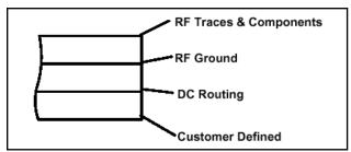
PCB dielectric between RF traces and RF ground layers should be chosen to reduce RF discontinuities between 50  $\Omega$  lines and package pins. M/A-COM recommends an FR-4 dielectric thickness of 0.008" (0.2 mm) yielding a 50  $\Omega$  line width of 0.015" (0.38 mm). The recommended metallization thickness is 1 oz. Copper.
