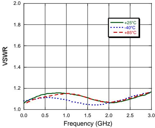
Input VSWR vs. Frequency over Temperature
