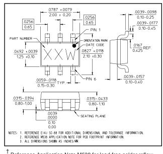
Reference Application Note M538 for lead-free solder reflow recommendations.
