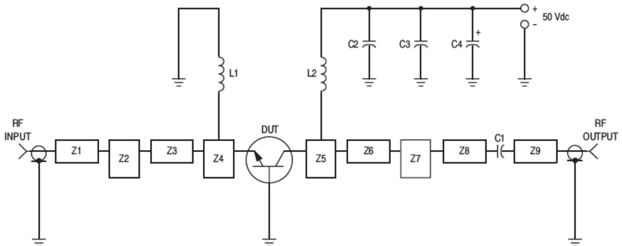
C1, C2 — 220 pF Chip Capacitor, 100-mil ATC
