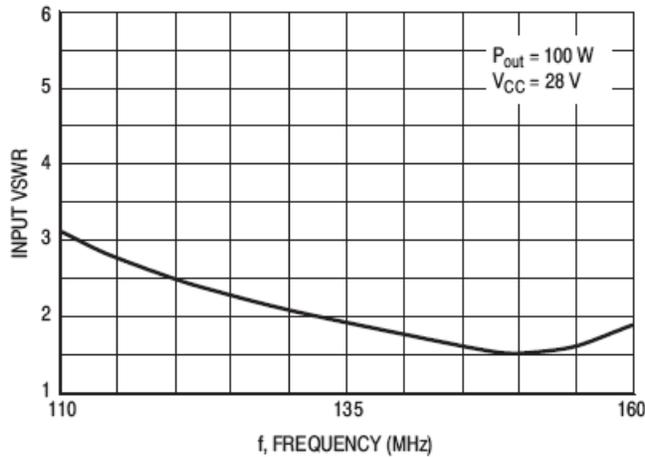
Figure 4. Input VSWR versus Frequency
