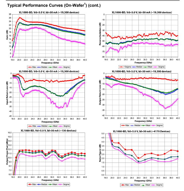
Note [1] Measurements – On-Wafer data has been taken using bias conditions as shown. Measurements are referenced 150 um in from RF In/Out pad edge. For optimum performance M/A-COM-Tech T-pad transition is recommended. For additional information see the M/A-COM-Tech "T-Pad Transition" application note.
