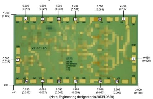
Units: millimeters (inches) Bond pad dimensions are shown to center of bond pad. Thickness: 0.110 + /-0.010 (0.0043 + /-0.0004), Backside is ground, Bond Pad/Backside Metallization: Gold All DC Bond Pads are  $0.100 \times 0.100$  ( $0.004 \times 0.004$ ). All RF Bond Pads are  $0.100 \times 0.200$  ( $0.004 \times 0.008$ ) Bond pad centers are approximately 0.109 (0.004) from the edge of the chip. Dicing tolerance: +/-0.005 (+/-0.0002). Approximate weight: 3.987 mg.
