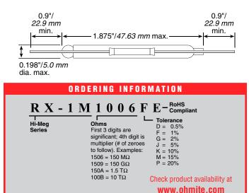
These Hi-Meg resistors are designed for use in electrometer circuits where a high order of performance is required. These resistors achieve a high degree of accuracy and stability, and operate at this high performance level for an extended period of time. By being vacuum sealed in a glass envelope, these Hi-Megs are suitable for ultra-high vacuum applications.
