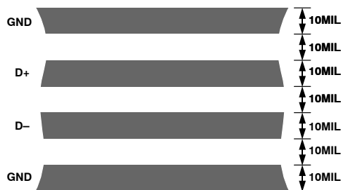
Figure 34. Arrangement of Signal Tracks
