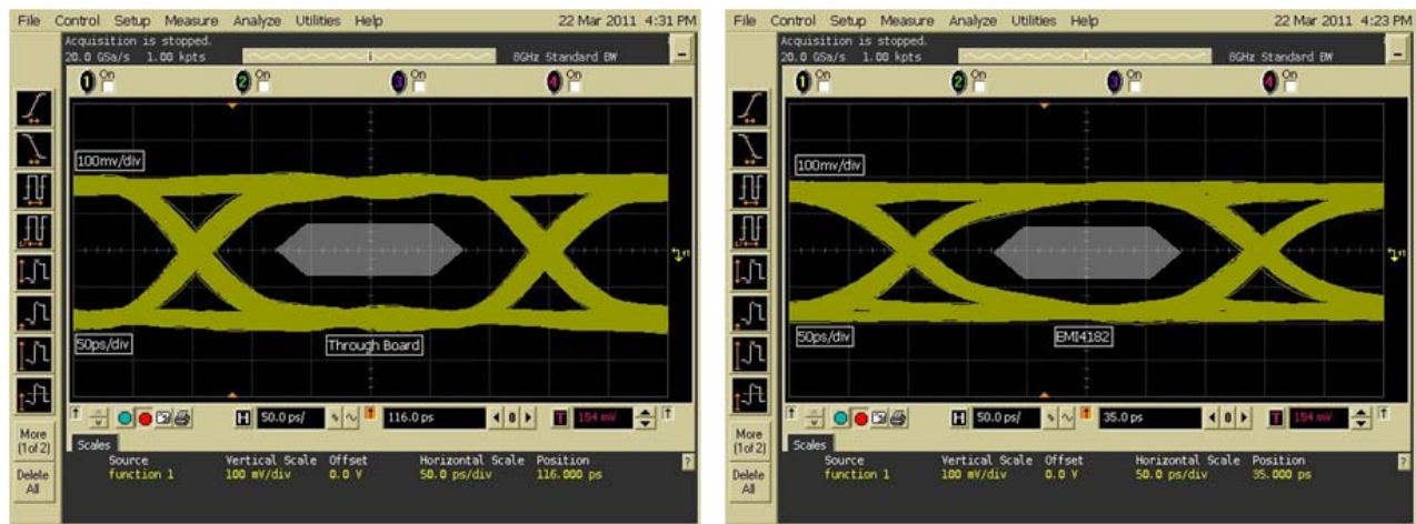
Figure 10. EMI4184 Measured Eye Diagram @ 3.4Gbps (EVB through on left, EVB with EMI4184 on right)
