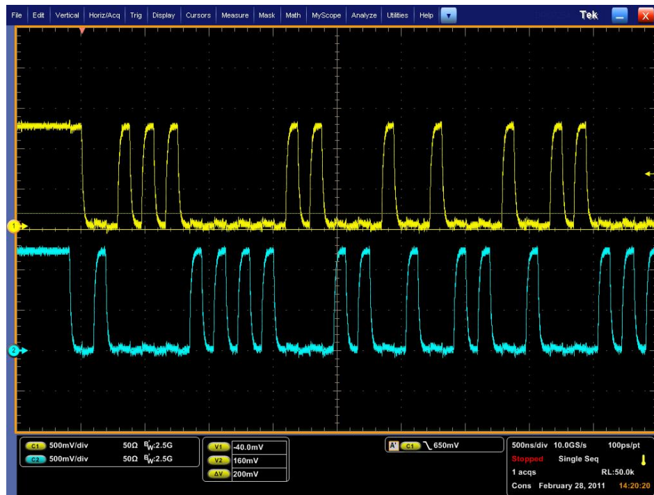
Figure 8. EMI4184 MIPI D-PHY LP Mode Measured Results
