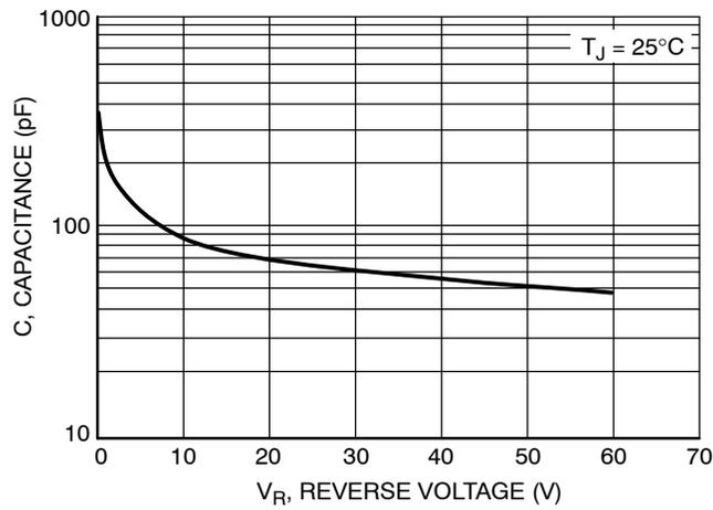
**Figure 7. Typical Capacitance**
