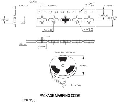
Example: ABC A=product type B=week code C=year code Reel: Terminal tape=40mm (min) Leader tape with empty cavities=350mm (min) Trailer tape with empty cavities=160mm (min) Devices per reel=1000
