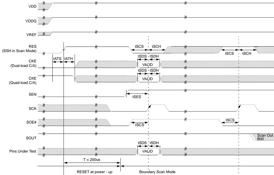
Note : To set the pre-defined ODT for C/A, a boundary scan mode should be issued after an appropriate ODT initialization sequence with RES and CKE signals
