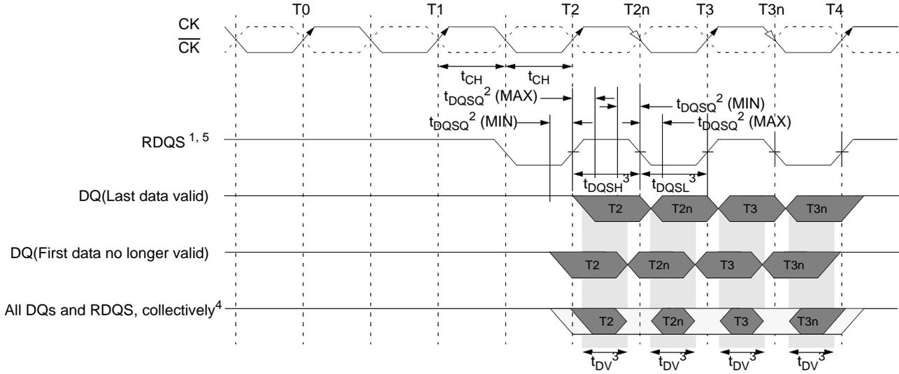
**Data Output Timing (2) -  $t_{DQSQ}$ ,  $t_{QH}$  and Data Valid Window**
