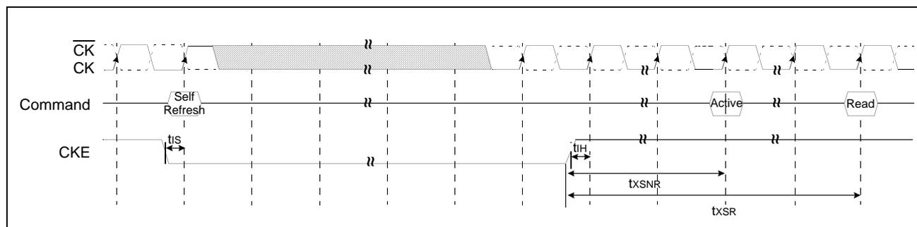
\* Once the device enters the self refresh mode, it should be in NOP state at least for 10ns. The minimum duration for the power down mode once CKE brought to down should be at least 10ns.
