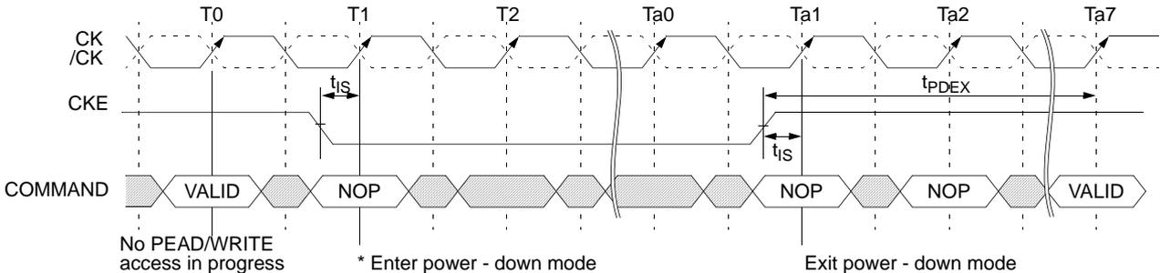
\* Once the device enters the power down mode, it should be in NOP state at least for 10ns. The minimum duration for the power down mode once CKE brought to down should be at least 10ns.
