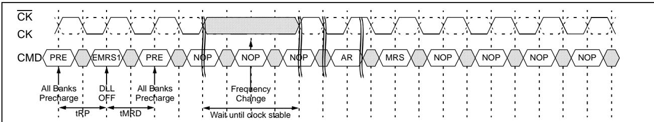
**Clock frequency change in case existing tCK is in DLL-off mode while desired tCK is in DLL-on mode**
