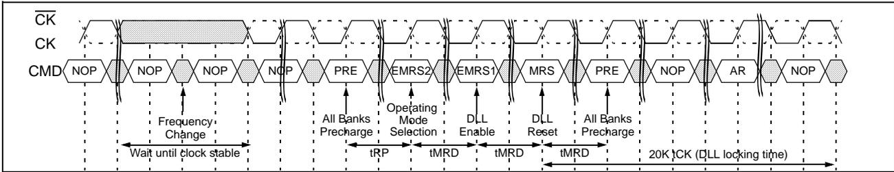
**Existing tCK is in DLL-on mode while desired tCK is in DLL-off mode**
