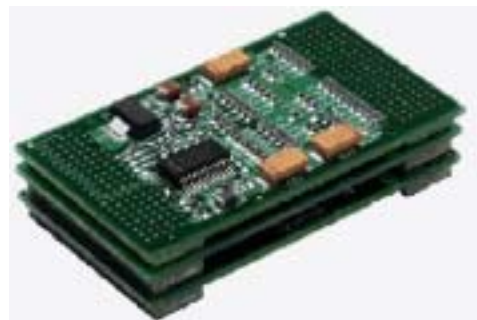
Figure 1 : NexMod Module shown with heat spreader removed
