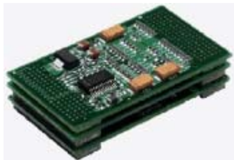
Figure 1 : NexMod Module shown with heat spreader removed
