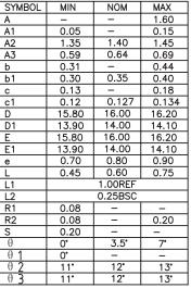
ALL DIMENSIONS MEET JEDEC STANDARD MS-026 BEB DO NOT INCLUDE MOLD FLASH OR PROTRUSIONS.
