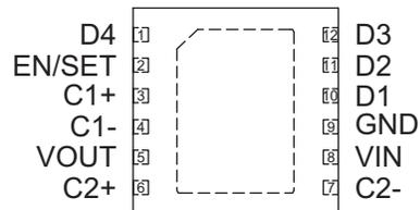
**High Efficiency 1X/1.5X/2X Charge Pump for White LED Applications****Absolute Maximum Ratings<sup>1</sup>**
