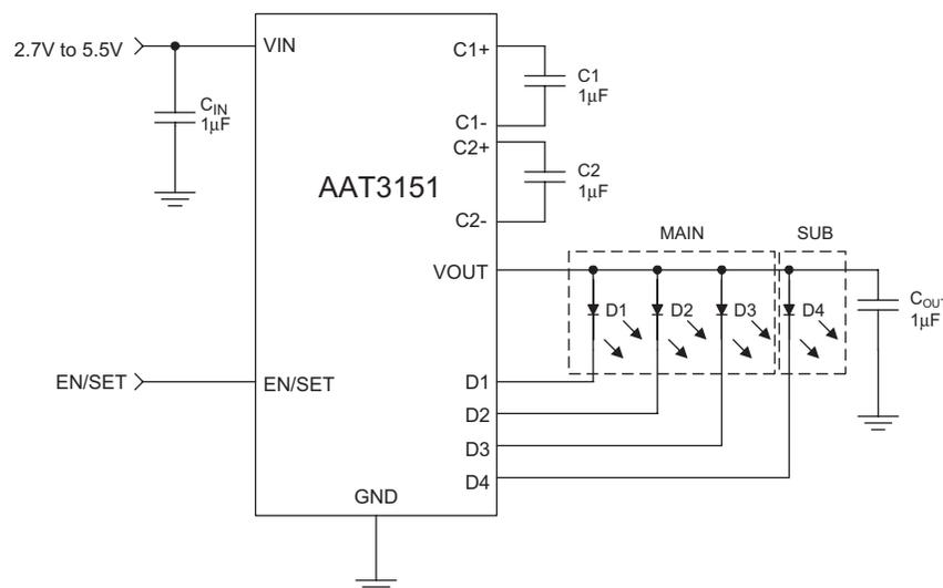
**AAT3151****High Efficiency 1X/1.5X/2X Charge Pump for White LED Applications****Pin Descriptions**
