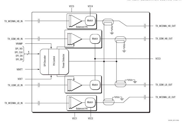
Figure 1. SKY77601 Functional Block Diagram
