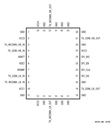
Figure 2. SKY77601 Pad Configuration – 34-Pin MCM (Top View)
