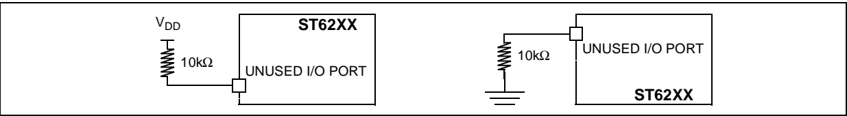
Figure 62. Two typical Applications with unused I/O Pin
