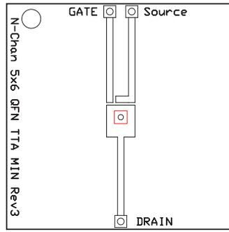
Max  $R_{\theta JA} = 118^{\circ}\text{C/W}$
