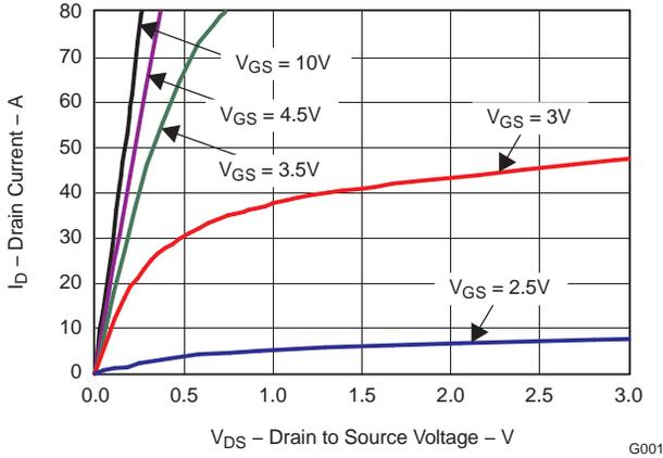
**Figure 2. Saturation Characteristics**
