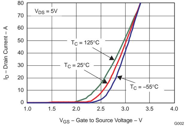
**Figure 3. Transfer Characteristics**
