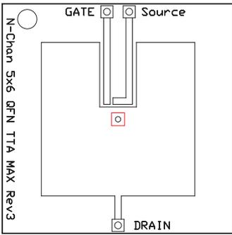
Max  $R_{\theta JA} = 51^{\circ}\text{C/W}$
