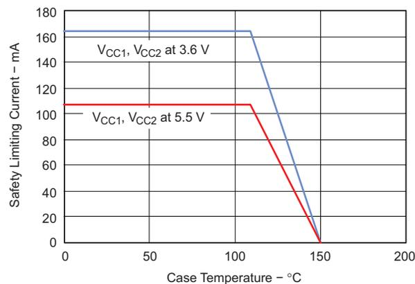
Figure 5. θ<sub>JC</sub> Thermal Derating Curve per IEC 60747-5-2
