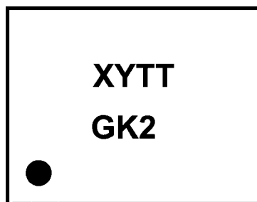
Top View XY - Date Code TT - Die Traceability G- Boomer K2 - LM49120TL
