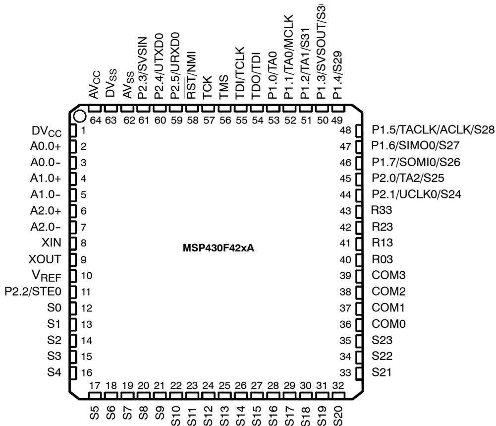
† It is recommended to short unused analog input pairs and connect them to analog ground.
