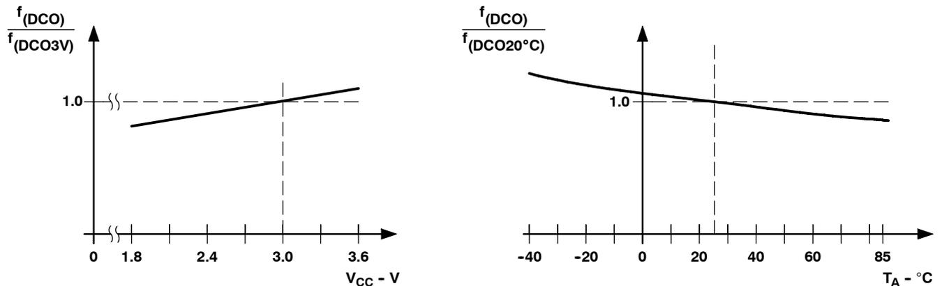
Figure 11. DCO Frequency vs Supply Voltage V<sub>CC</sub> and vs Ambient Temperature
