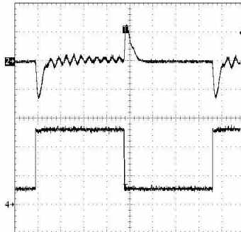
Figure 20. Overcompensated (Damped Oscillation), R_C Is Too Large
