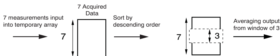
Figure 28. MAV Filter Operation (Patent Pending)
