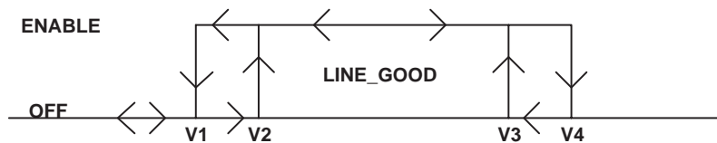
Figure 2. Line UVLO and OVLO Operation
