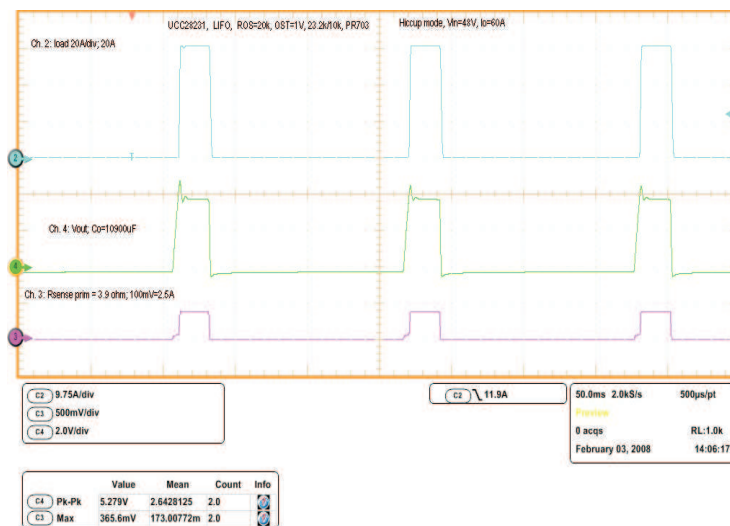
Figure 42. Cycle-by-Cycle Current Limit
