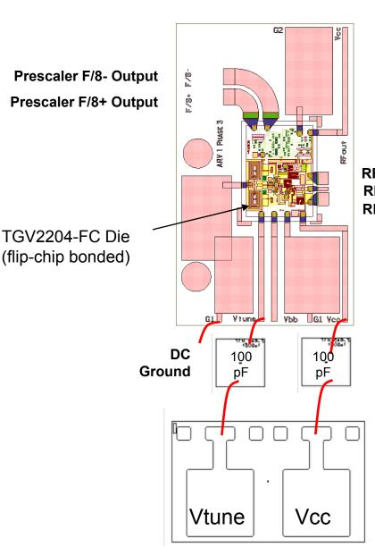
Alumina substrate board Thickness: 0.38 mm  $\varepsilon_r = 9.9$
