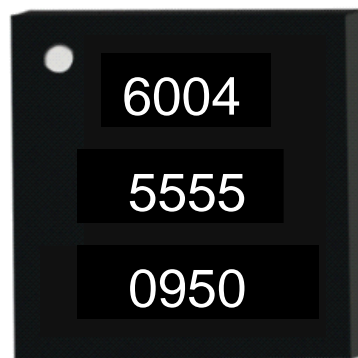
16-lead QFN 4 x 4 mm
