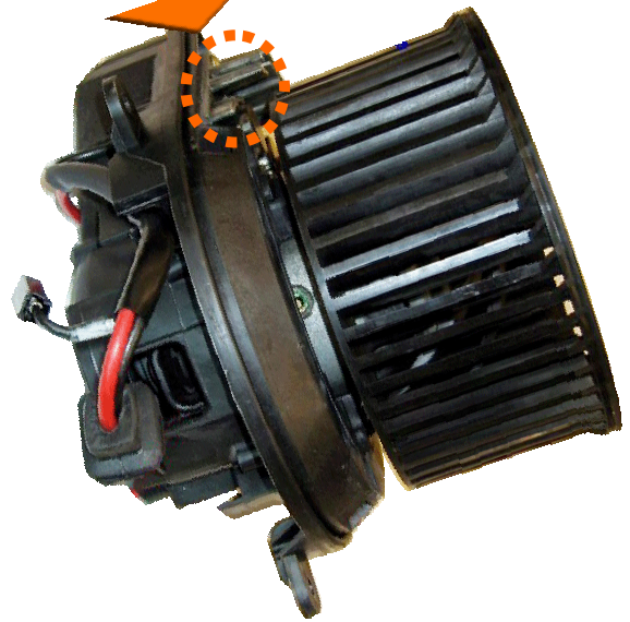
CAR Blower Speed control
