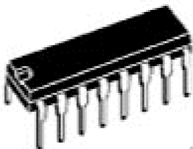
DIP Dual Inline Package
