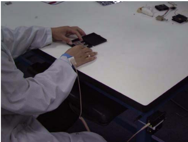
Proper buttoning of smock. The bottom button (although a little hard to see) is buttoned.
