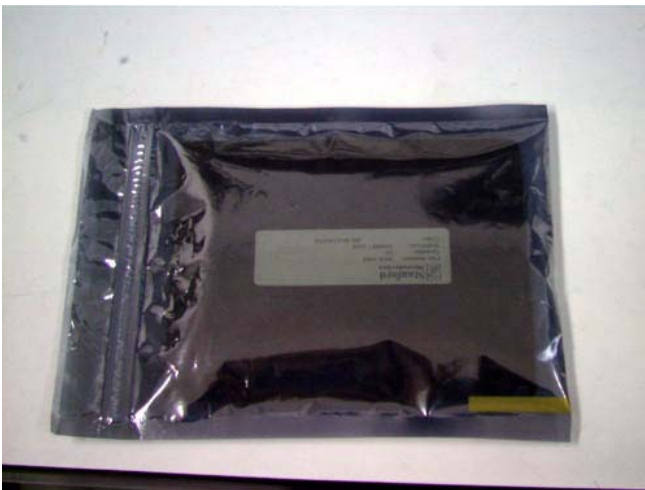
Static shielded bags are typically dark silver in color, and may (or may not) have the ziplock mechanism on them. They should be marked as "static shielded" somewhere on the surface of the bag. These are highly recommended for transporting static sensitive devices.
