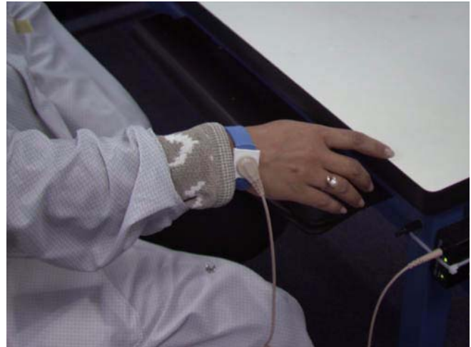
Improper coverage of personal clothing. Notice the exposed sleeve visible due to improper smock sizing or operator error.
