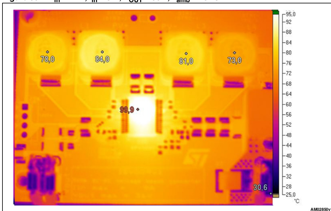
Figure 40. V_{in} = 24\text{ V} , I_{in} = 8\text{ A} , V_{OUT} = 26\text{ V} , T_{amb} = 25\text{ }^{\circ}\text{C}
