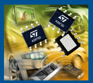
A597x family is composed of seven monolithic step-down switching regulators capable of delivering more than 2 A. They are housed in small outline packages such as S0-8, qualified following the AEC-Q100 requirements (Product Part Approval Process available).
