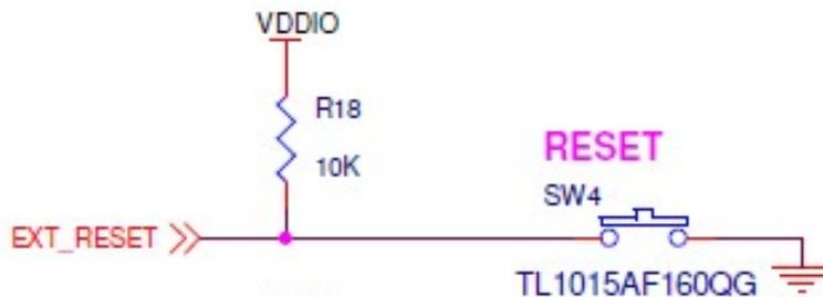
EXT\_RESET signal is active low signal (active or asserted state occurs when the signal is at a low voltage level).
