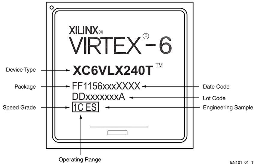
Figure 1: XC6VLX240T-1FF1156CES Marking
