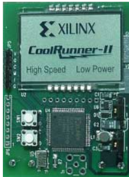
Figure 1: CoolRunner-II Demo Board
