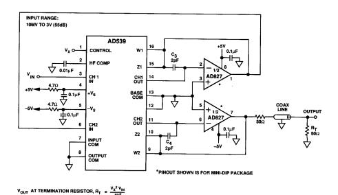
$V_{OUT}$  AT PIN & OF AD827 =  $\frac{V_{\chi^2} V_{IN}}{4V^2}$
