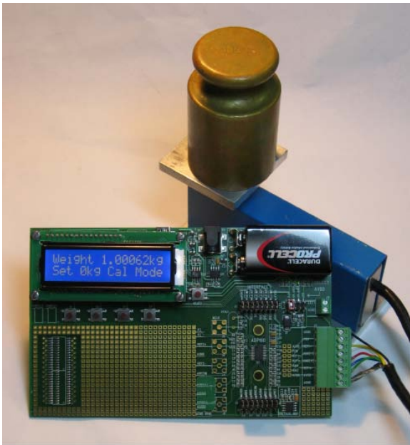
Figure 2. Weigh Scale System Using the AD7191
