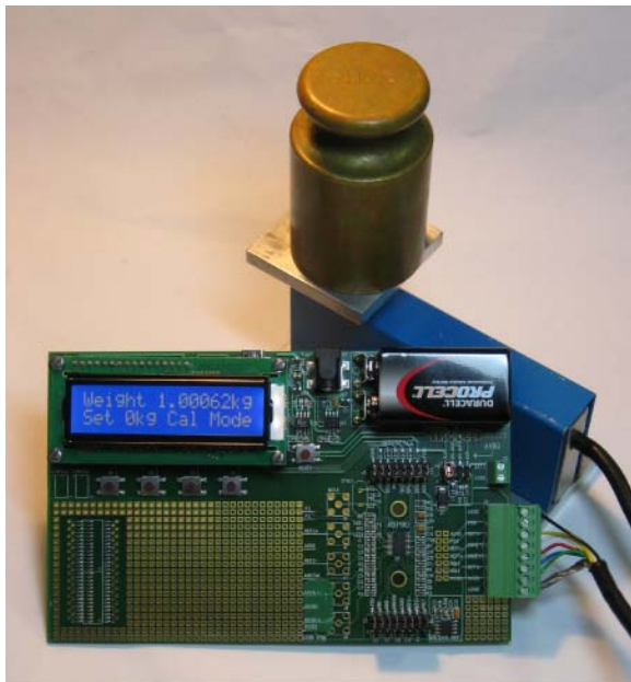
Figure 2. Weigh Scale System Using the AD7192
