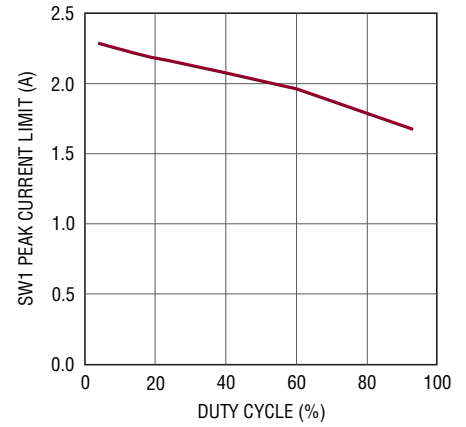
HV Channel Current Limit vs Duty Cycle
