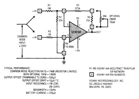
Figure 1.  $\pm 250$ V Common Mode Range Instrumentation Amplifier (A<sub>V</sub> = 1)
