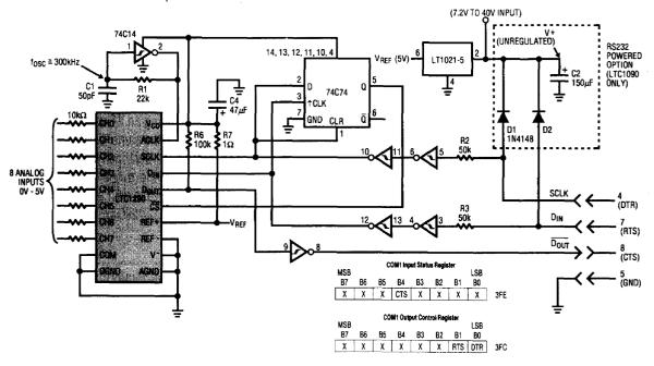
Figure 1. LTC1290 to IBM PC Serial Port Interface
